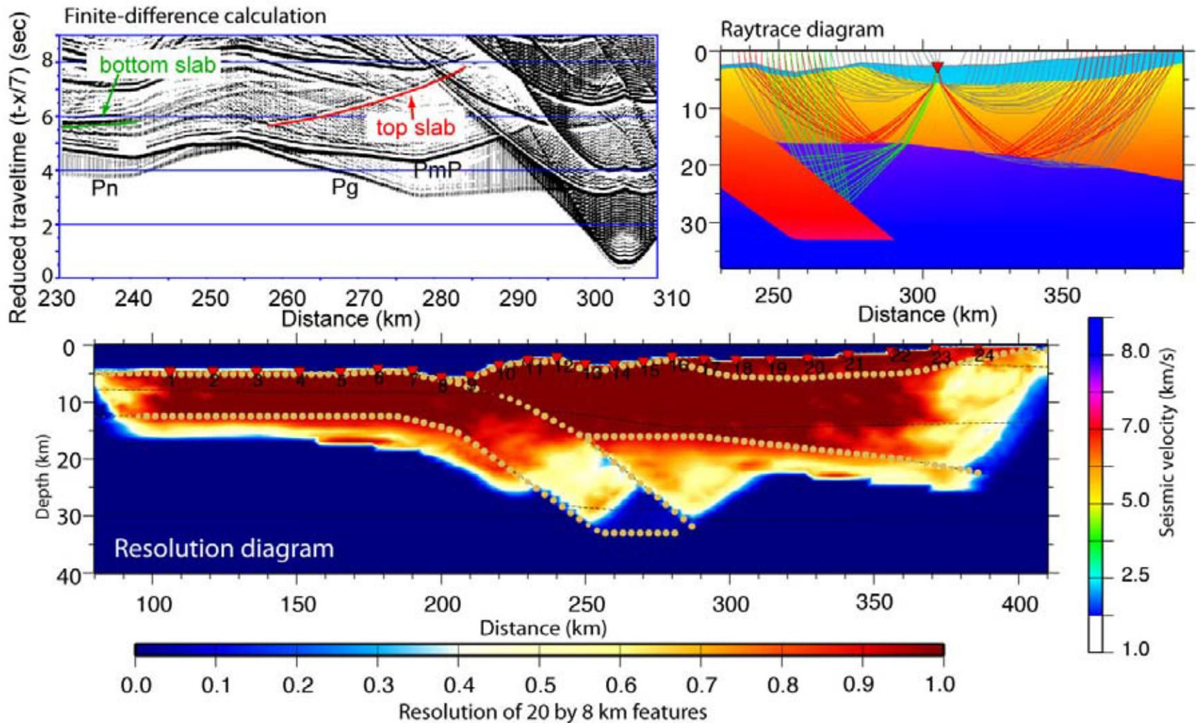
Depending on data quality, deep structure can be imaged with first-arriving phases, or with a combination of later phases in the wide-angle data.
