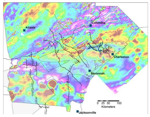
Figure 1. Location map of the South Georgia Rift (SGR) basin (light gray contour, after Chowns and Williams, 1983) in South Carolina and Georgia superimposed on the magnetic anomaly map. Existing deep seismic lines (USGS and COCORP) are shown as black lines together with newly acquired 2-D seismic lines (6 s TWT in bold) as part of the DOE  $CO_2$  sequestration project.
