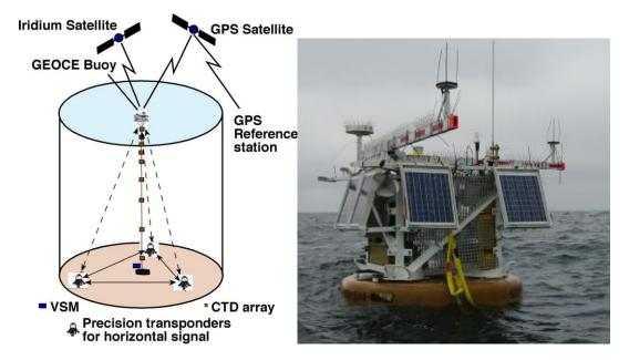
Figure 2: Moored-buoy for continuous horizontal and vertical deformation measurements: concept (left), implementation (right).
