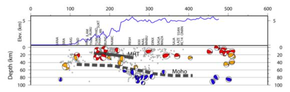
Figure 7. Cross section showing seismicity and focal mechanisms. Grey lines denote Main Himalayan Thrust (MHT) and the Moho from Schulte-Pelkum et al. (2005). Regional topography is plotted above the seismicity with approximate locations of the HIMNT stations.
