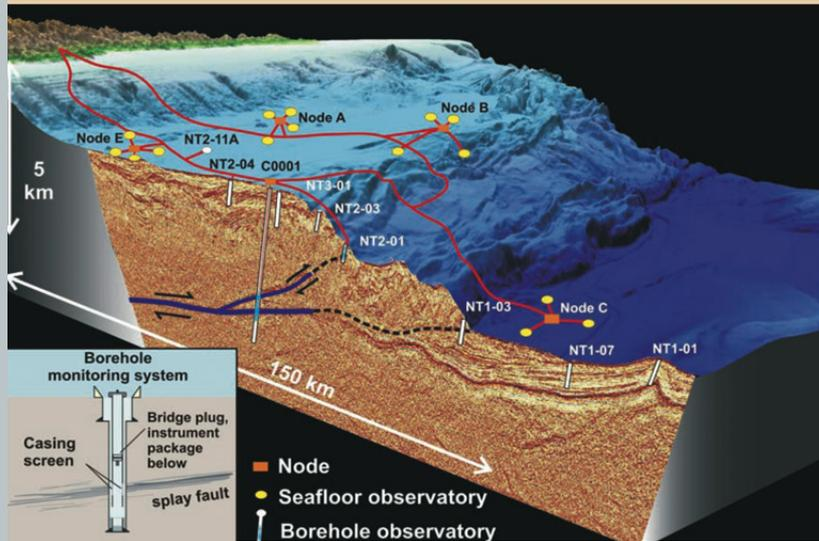
DONET cabled observatory network in the Nankai Subduction zone: calibration and verification of models, monitor and sampling, active perturbation experiments, early warning system
