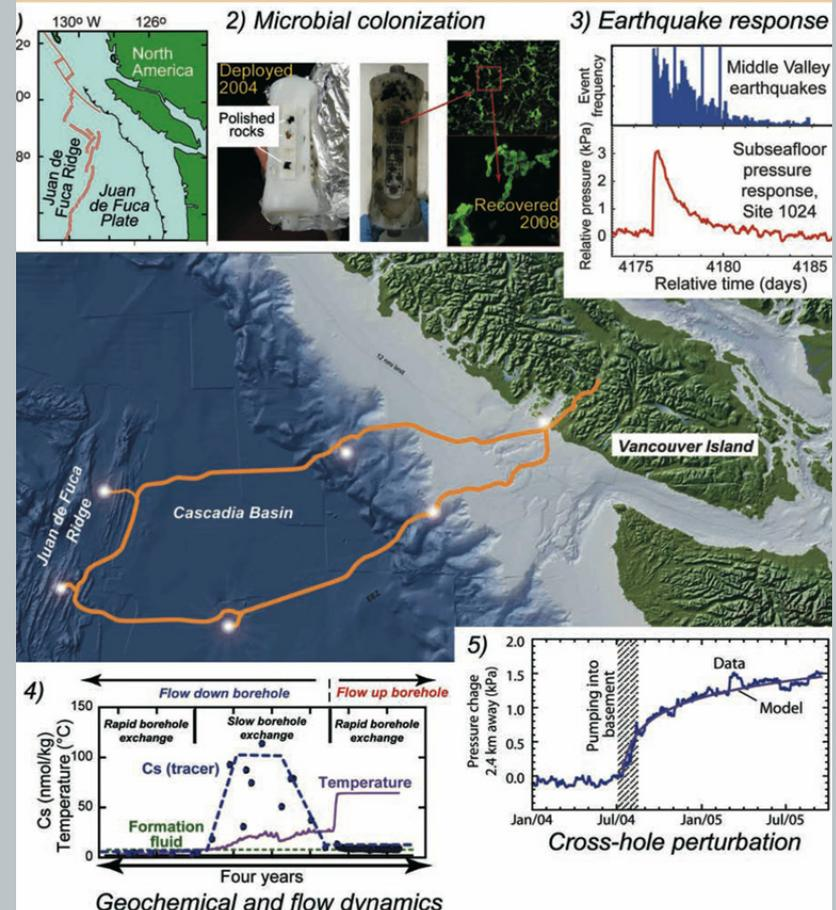
Linking lithospheric, hydrogeologic and microbial systems- Planned network at NEPTUNE Canada
