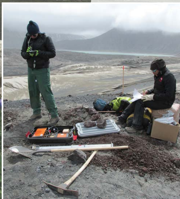
Seismic station being installed inside Okmok caldera
