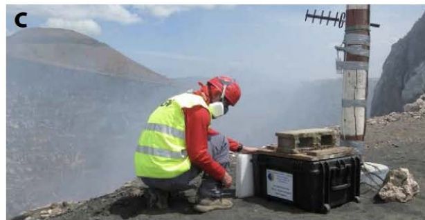
(C) Deployment of a multi-gas sensor at Masaya Volcano, Nicaragua, as part of the Deep Carbon Observatory's DECADE initiative. Photo credit: Alessandro Aiuppa and Marco Liuzzo (INGV)
