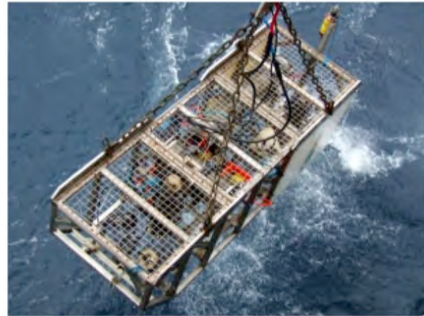
SHRIMP – deep towed camera platform, up to 5000 m
