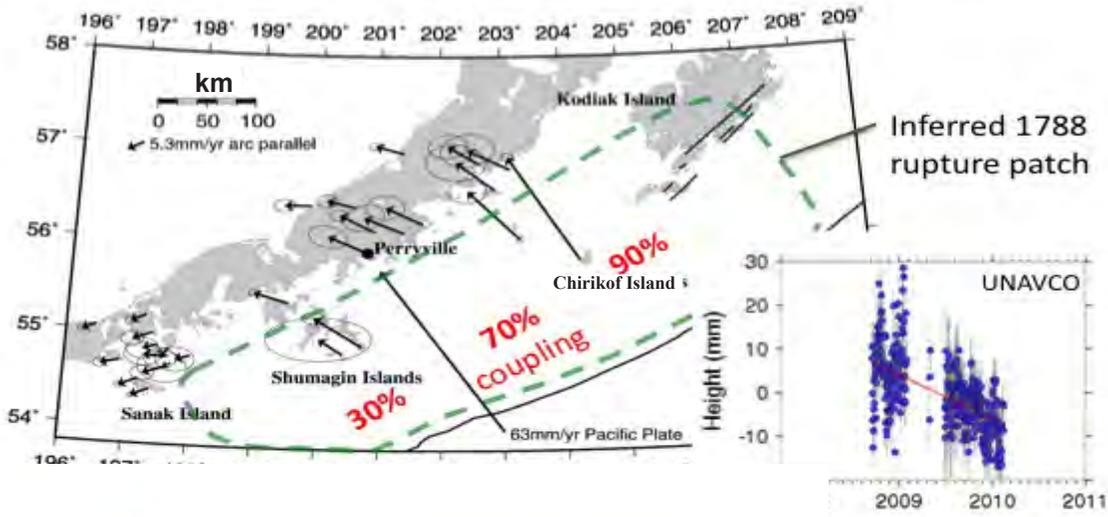
Figure 1. GPS velocities relative to the Pacific plate for sites in the eastern Aleutians (Fournier and Freymueller, 2007), UNAVCO vertical GPS velocities from Chirikof Island (inset) showing  $\sim 10$  mm/yr subsidence of the island, and a possible rupture area for the great 1788 earthquake inferred from minimum tsunami heights recorded by Russian settlements. Chirikof Island lies above a highly coupled section of the megathrust.
