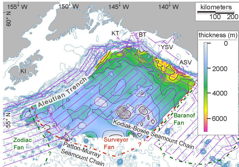
Figure 1. Two-way travel time thickness map of the Surveyor Fan. Seismic reflection data tracklines used in calculation shown in purple. Estimated boundaries of the Surveyor, Zodiac, and Baranof Fans shown in red and green dashed lines, respectively. ASV- Alek Sea Valley; BT- Bering Trough; KI- Kodiak Island; KT- Kayak Trough; YSV- Yakutat Sea Valley. (Reece et al., 2011).
