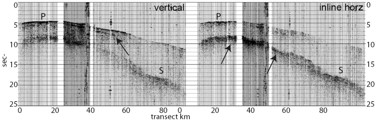
Figure 2. Local earthquake collected into SAHKE transect. 3-C stations have 300 m spacing with 150 m densification in the middle. Magnitude 2.0 earthquake is at 26 km depth, just above the slab interface. Sharp secondary P event may be associated with interface or subduction-related structure at base of overlying plate. S-waves exhibit lateral variation in first and secondary (coda) waveform character. Heterogeneity in overlying plate affects arrival times.
