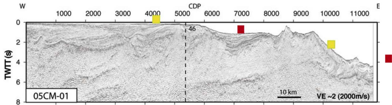
Figure 3. Proposed location of GPS-Acoustic sites of the southern transect along seismic reflection profile in the Hawke Bay area (Bell et al., 2010). See Fig. 1 left for transect location. Red and yellow indicate primary and secondary sites, respectively, as explained in the text.
