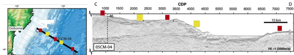
Figure 2. Proposed location of GPS-Acoustic seafloor sites of the northern transect along reflection profile offshore of Gisborne (Bell et al., 2010). Left shows map view, right shows profile. Red and yellow indicate primary and secondary sites, respectively, as explained in the text.
