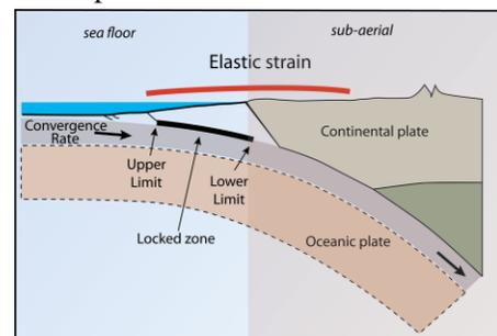
Figure 1: Subduction Profile showing offshore and onshore strain.
