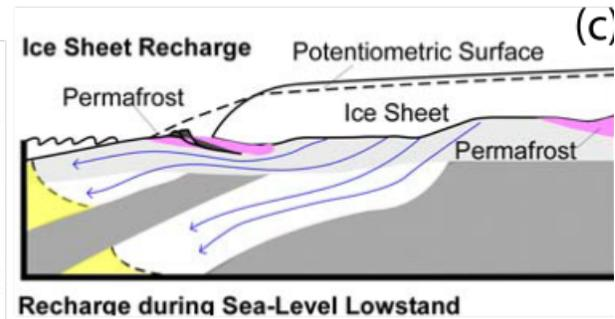
Fig 2. Example of impacts of glacial loading on submarine groundwater systems (blue arrows) including extending the freshwater zone and changing location and chemistry of SGD.
